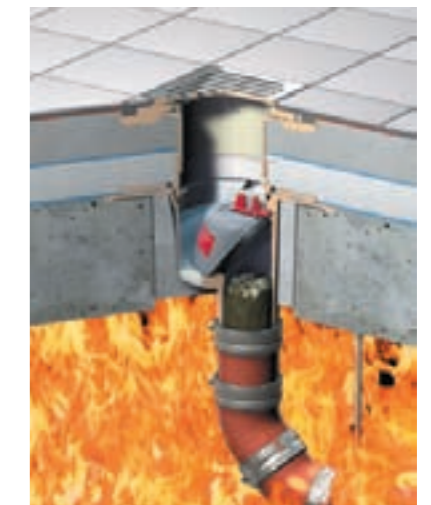
A fire on top of the ceiling expands. The intumescent mass in the odour seal to completely block the drain
