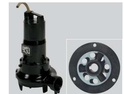
SITA submersible pump. The laterally inset vortex wheel (right) guarantees complete diameter flow. It is therefore also suitable for fibrous and contaminated wastewater
