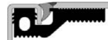
Installation example: Sealing vinyl sheet flooring against drainage channels and gullies
